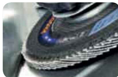
Inefficient, because most of the abrasive material remains unused
